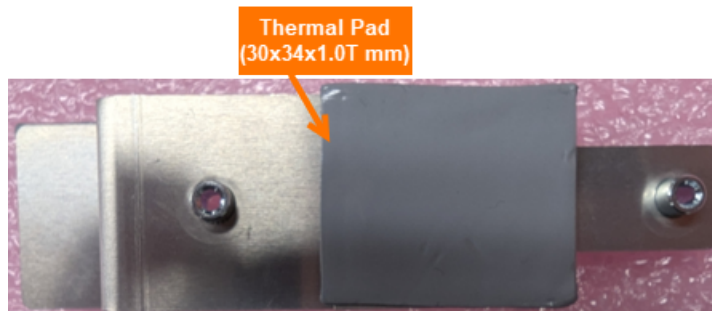
Figure 2-5 Thermal pad (18x30x1.0T mm) attached to the heatsink
