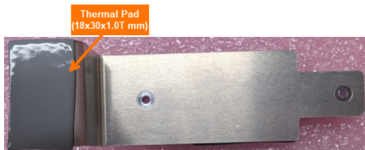
Figure 2-5 Thermal pad (18x30x1.0T mm) attached to the heatsink
